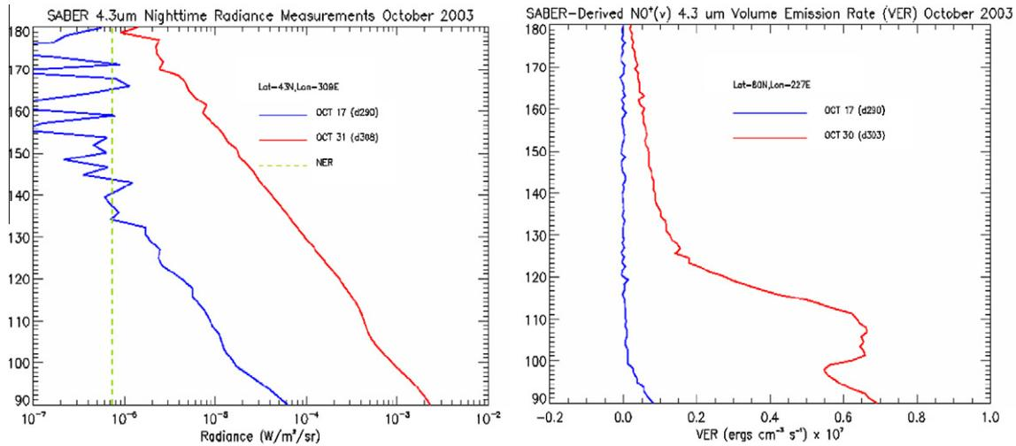
Fig. 2. Nighttime radiance and VER measurements before (blue line) and during (red line) Halloween 2003 magnetic storm. (For interpretation of the references to color in this figure legend, the reader is referred to the web version of this paper.)
