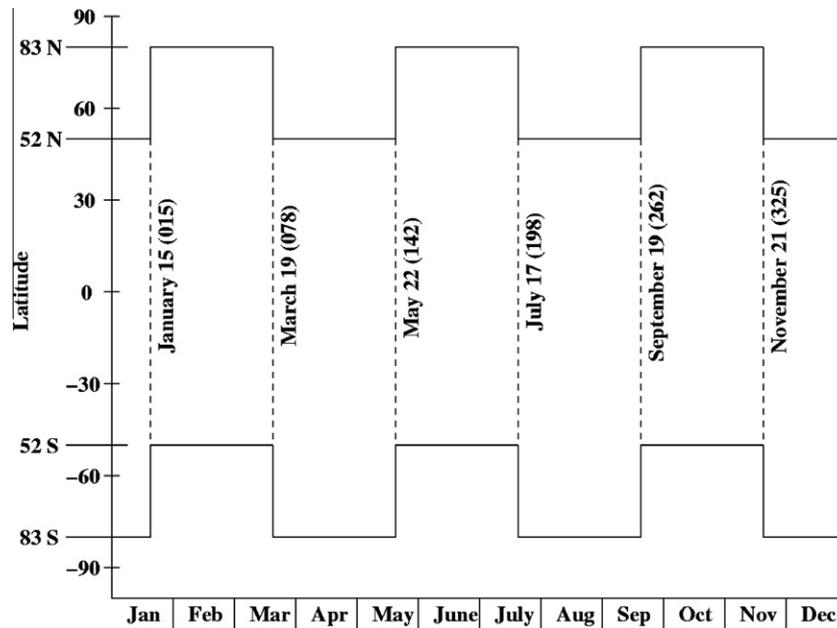
Fig. 1. TIMED/SABER latitude coverage during 2003. Dashed line indicates the yaw maneuvers.
